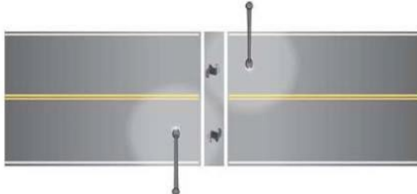
Figure 6.5 Crosswalk Lighting Pole Placement
