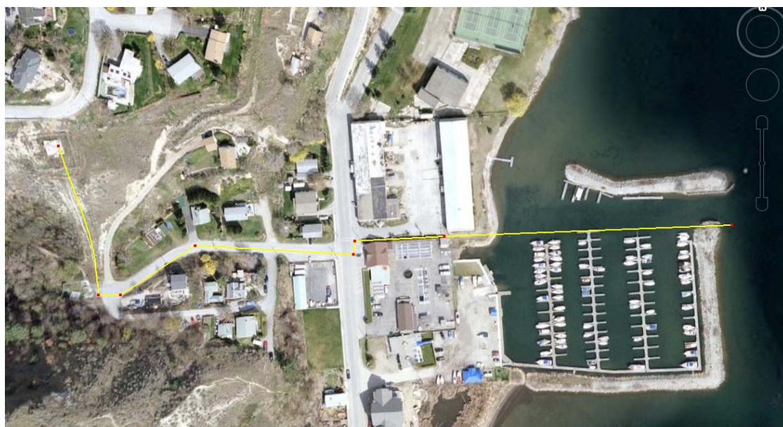
50,000 US gallon Reservoir located at elevation 384.10 (slab). HWL = 387.08 m (Yellow line denotes watermain) Emergency use only. Capacity in the course of a year with 400 USgpm running for 4 months, 265 ML
