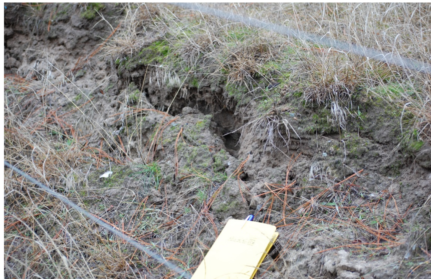
Photograph 3837: Looking southwest at fresh tension crack along slide head scarp where horizontal and vertical displacements of 10 to 15 cm exist within natural sand deposits.
