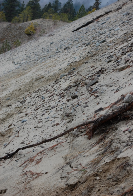
Photograph 3882 (left): Looking southwest along mid slope at recent tension crack (partially obscured by ravelled material) across sand and gravel face overlooking lower slide bench. Lack of grass, shrubs or small tree cover is indicative of ongoing raveling from continuing creep movements.
