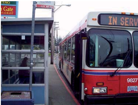
Misplaced sign, shelter obstructs sidewalk
