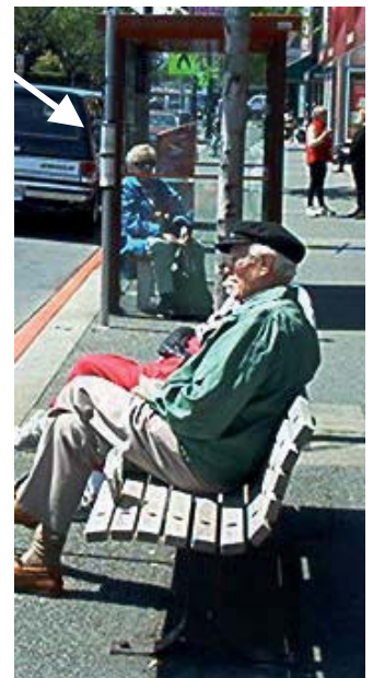
Shelter openings should face the bus. This shelter is turned around – passenger has her back to the bus.
