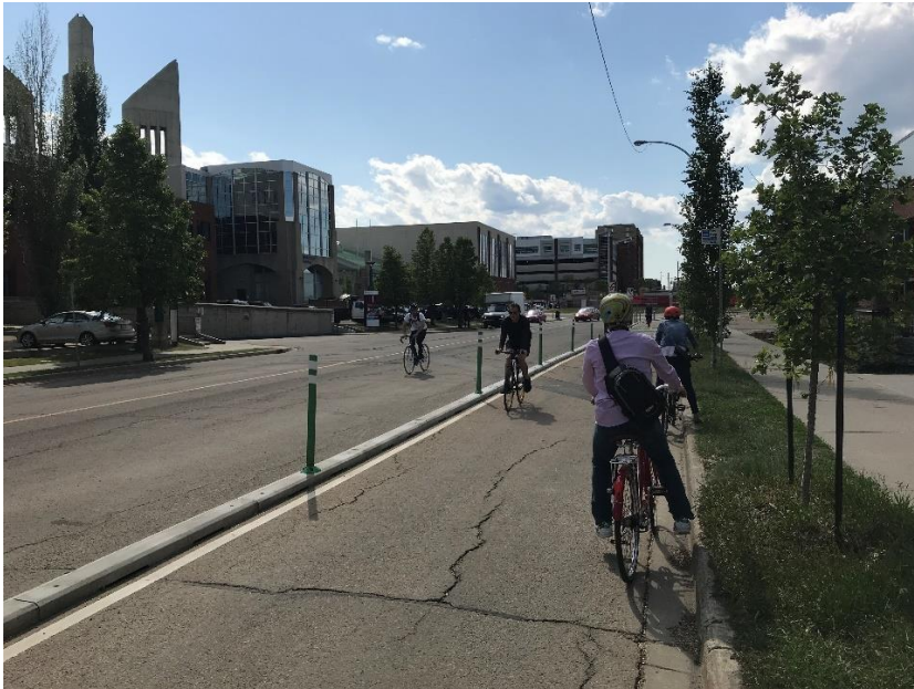
Figure 11. Bidirectional Protected Bicycle Lane
