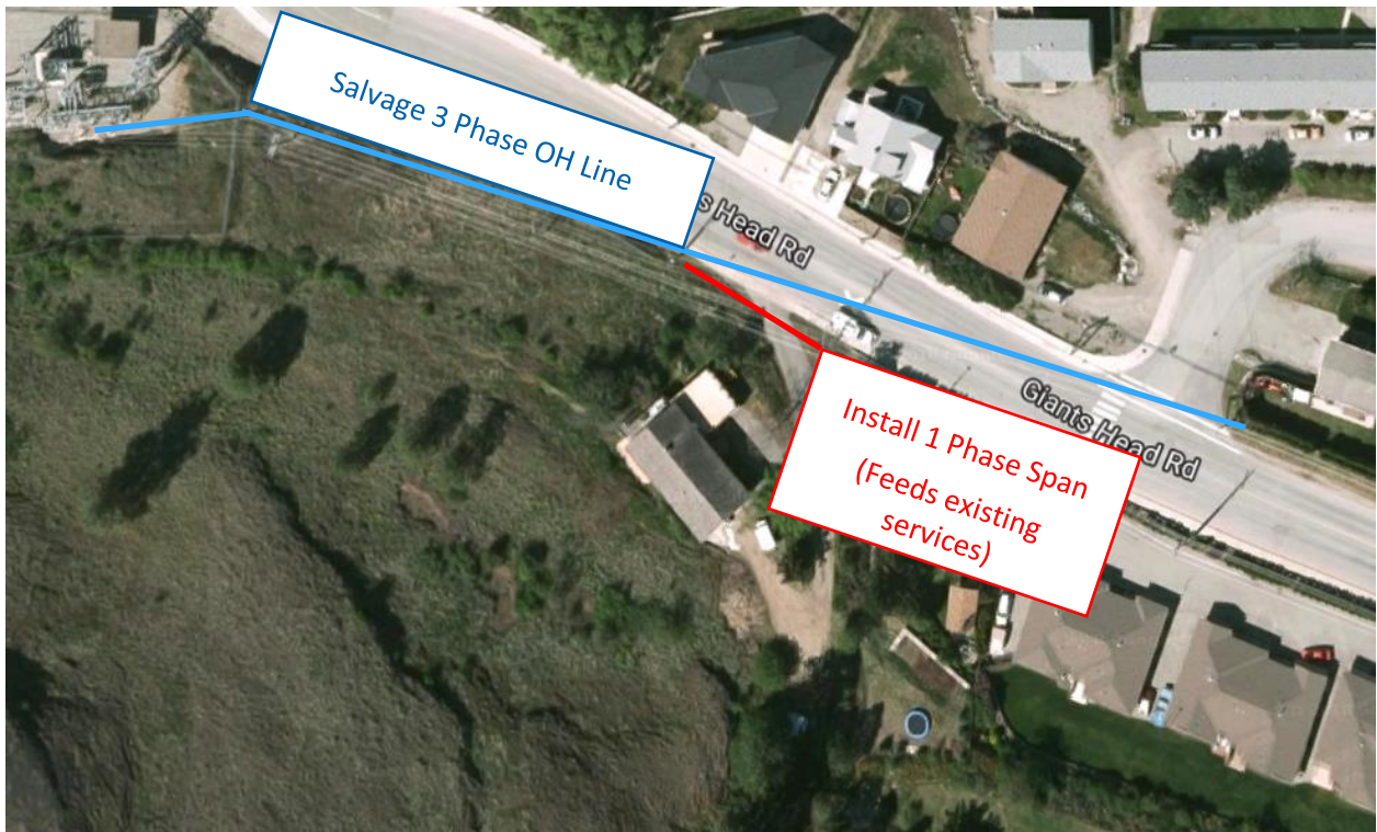
Figure 30: Salvage of feeder 249 egress
