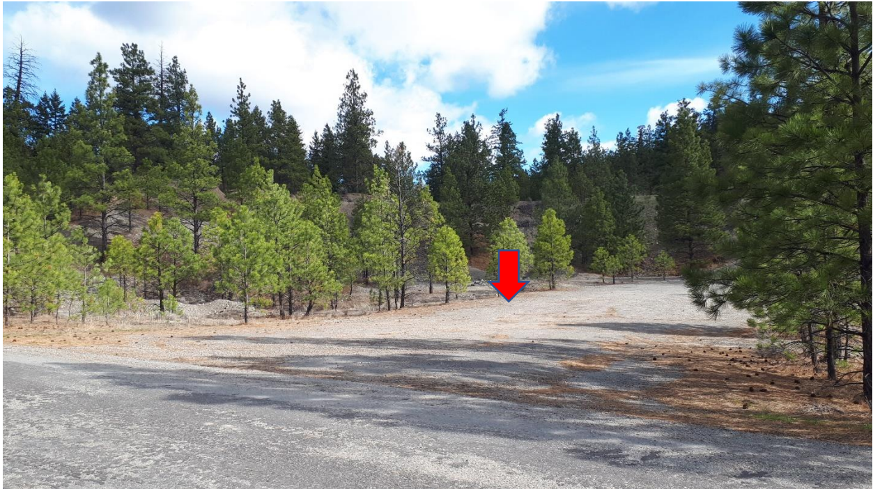
Photo One. Looking north-east at the main gravel extraction area for the site. The upper bench in the background once spanned out into this excavated area to approximately where the red arrow has been positioned.
