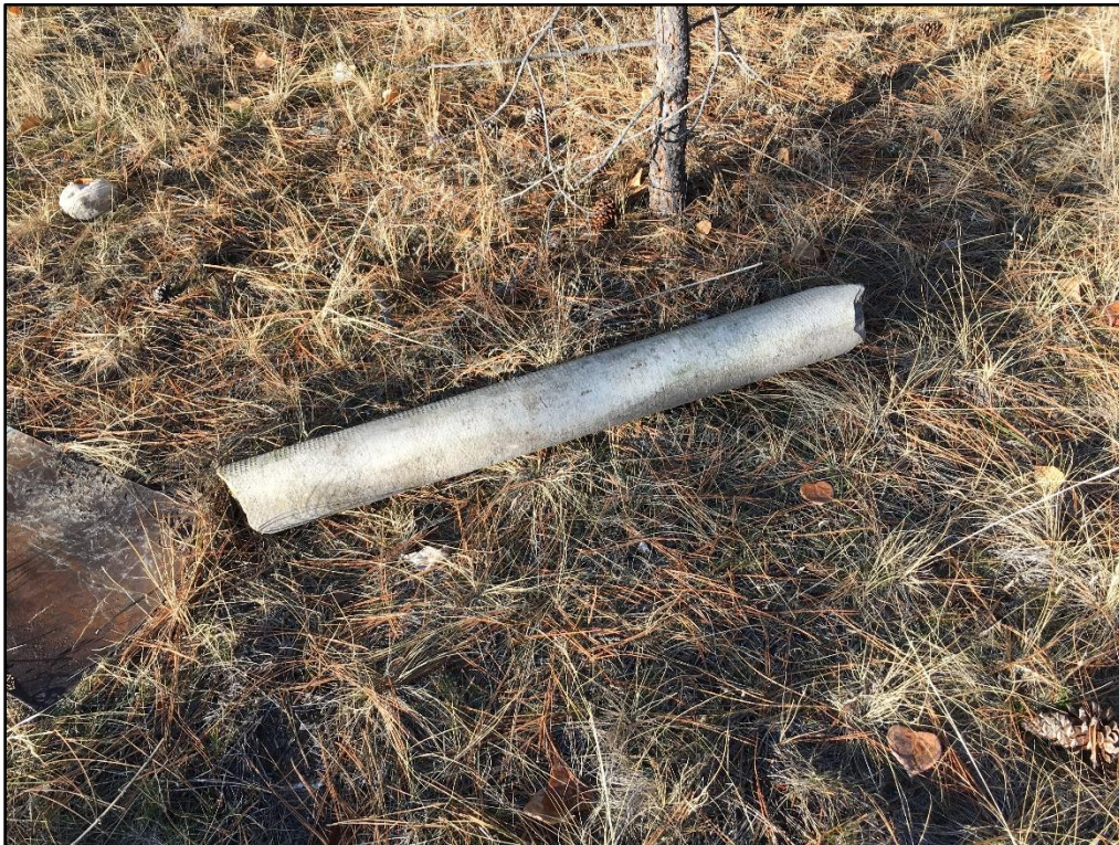
Photograph 4: View of an Asbestos Cement Pipe in APEC #1 (November 30, 2019).
